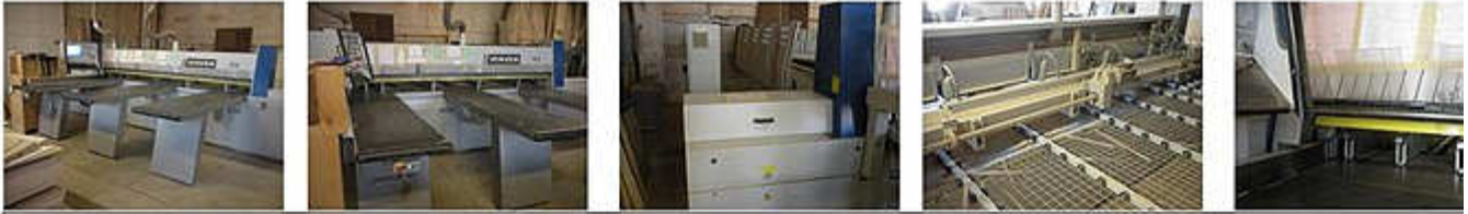
MEYER PS-8 3200MM 10' Panel Saw 2003 Model 3200mm 10' Cutting Length 80MM Finish Cutting Height 20 H.P. Main Motor 1.5 H.P. Scoring Motor Side Pressure Device for Squaring Crosscut Parts 5 -100 MPM Saw Carriage Forward 130 MPM Return Electronic Cutting Height Option Grooving
