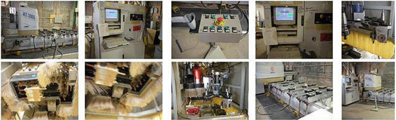
BUSELLATO JET 3000 Point to Point Machining Center 2000 Model Useful Working Field 120.1" X 48" X 7.5" Positioning Speeds "X" 70MPM "Y" 61 "Z" 12 MPM Genesis Software 6 Rails with 21 Pods Panel Lifters TF17 Boring Head with 10 on "X" and 7 in "Y" 2+2 Horizontal 12.5 H.P. Electric with 0-360 Degree CNC Unit 8 Position Tool Changer Auxiliary 9.5 H.P. Router ISO-30 Tool Interface "Autolink" Seamless Link and Base Software with Scanner Saw / Router Aggregate Manually Adjustable
